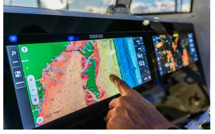
introduced a unique GPS chartplotter combo screen, the NSX Ultrawide. It offers the same active area as two smaller displays, but in terms of functionality it offers so much more. The screen is 14.5" diagonal but only 7" high,
